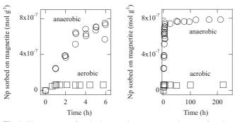
**Fig. 1.** The amount of sorbed neptunium on magnetite as a function of time at pH = 5.7 to 5.9 in 0.1 mol L<sup>-1</sup> NaNO<sub>3</sub> solution under aerobic and anaerobic conditions. The initial concentration of Np(V) is  $1.8 \times 10^{-5}$  mol L<sup>-1</sup>. The amount of magnetite is 1 g and volume of liquid phase is 50 mL.
