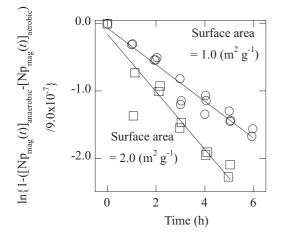
**Fig. 4.** The amount of sorbed neptunium on magnetite (surface area was 1.0 and  $2.0 \text{ m}^2 \text{ g}^{-1}$ ) as a function of time at pH = 5.7 to 5.9 in 0.1 mol L<sup>-1</sup> NaNO<sub>3</sub> solution under anaerobic condition showed by  $\ln\{1 - ([Np_{mag}(t)]_{anaerobic} - [Np_{mag}(t)]_{anaerobic})/9.0 \times 10^{-7}\}$  versus time. The initial concentration of Np(V) is  $1.8 \times 10^{-5} \text{ mol L}^{-1}$ . The amount of magnetite is 1 g and volume of liquid phase is 50 mL.
