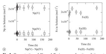
**Fig. 3.** Concentration of Np and Fe ions as a function of time at pH = 6.0 in  $0.1 \text{ mol } L^{-1} \text{ NaNO}_3$  solution under aerobic condition. The initial concentration of both Np(V) and Fe(II) are  $2.2 \times 10^{-6} \text{ mol } L^{-1}$ . (a) Concentration of Np(V)–Np(IV), (b) Concentration of Fe(II)–Fe(III).
