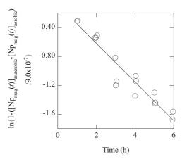
**Fig. 2.**  $\ln(([Np_{mag}(t)]_{anaerobic} - [Np_{mag}(t)]_{anaerobic})/9.0 \times 10^{-7})$  versus time under anaerobic condition. Initial concentration is  $1.8 \times 10^{-5} \text{ mol } \text{L}^{-1}$
