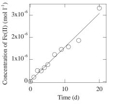
**Fig. 5.** The concentration of Fe(II) ion dissolved from magnetite (surface area was  $1.0 \text{ m}^2 \text{ g}^{-1}$ ) as a function of time at pH = 6.0 in 0.1 mol L<sup>-1</sup> NaNO<sub>3</sub> solution under anaerobic condition. The amount of magnetite is 2 g and volume of liquid phase is 100 mL.
